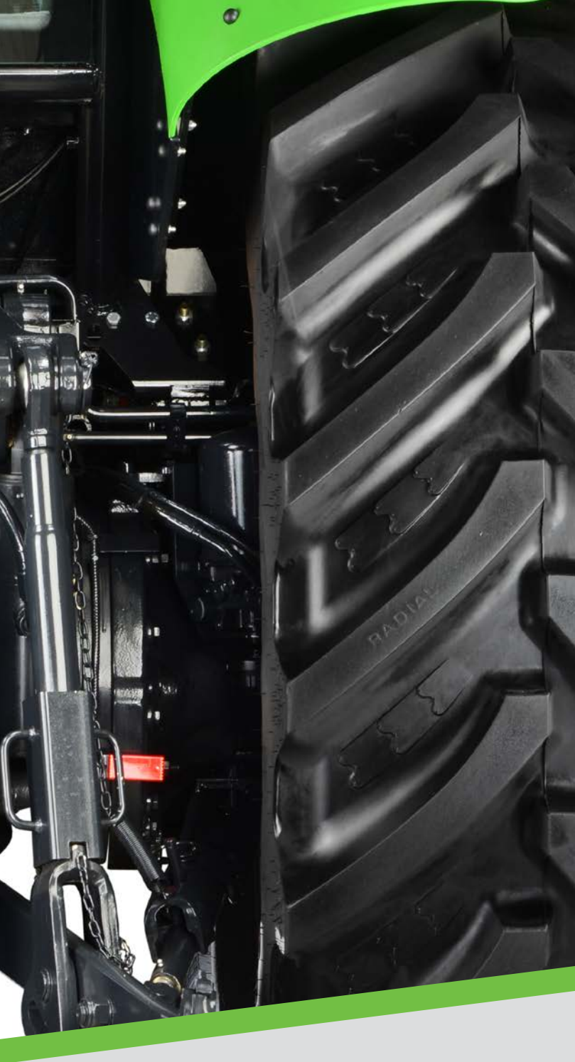
External rear lift and PTO remote controls from each side.
