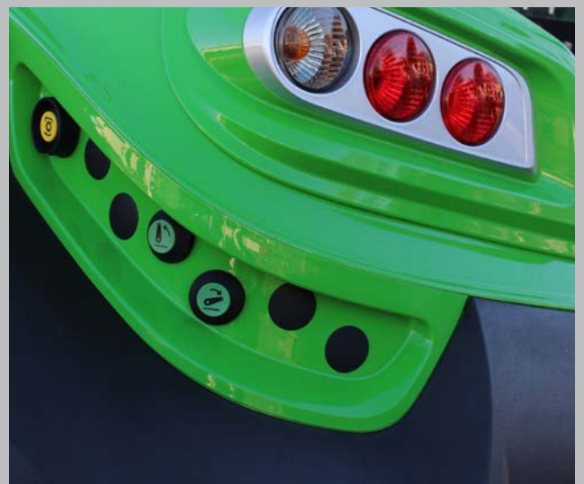
External rear lift and PTO remote controls from each side.
